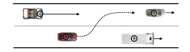
As such, the AdCoS requires the integration of MTTs for context assessment that are able to provide context-dependent estimations about the current lane-change intentions of the human driver. Within the AdCoS "Adapted Assistance", this ability is provided by the **Driver Intention Recognition** (DIR) module.
